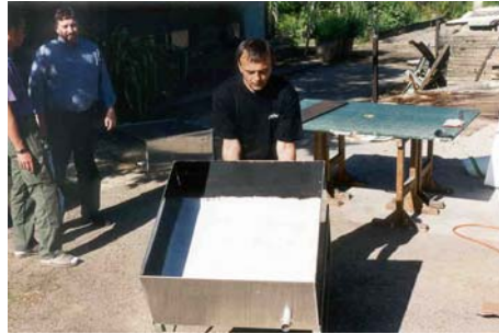
GEISENHEIM, JUNE 1996, PREPARATION OF THE CONTAINERS FOR THE ANTI-ROOT TEST
