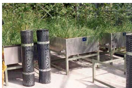
PLANTS WITH AGGRESSIVE ROOTS USED FOR THE ANTI-ROOT TEST
