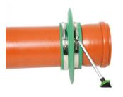
Use a screwdriver to tighten the clamping straps sufficiently to prevent the **RONDO Sealing collar** from shifting during concreting.
