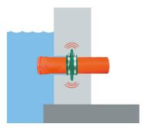
Der **RONDO Sealing collar** is placed in center of the concrete element.
